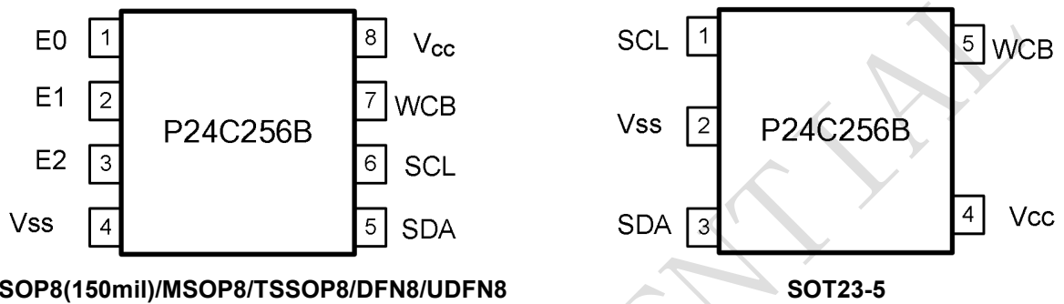
Figure 1-1 Pin Configuration
